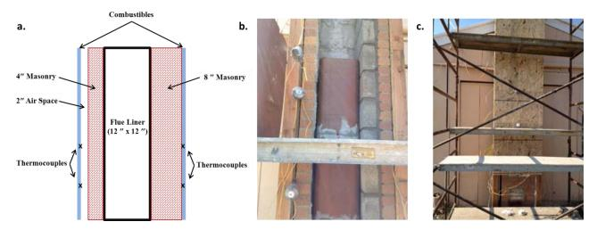
Figure 2 – (a) Diagram of the Chimney Test Configuration, (b) Photograph of the Test Chimney to Show the Masonry Configuration and (c) a Photograph Showing the Final Appearance after a Plywood Enclosure was Installed
