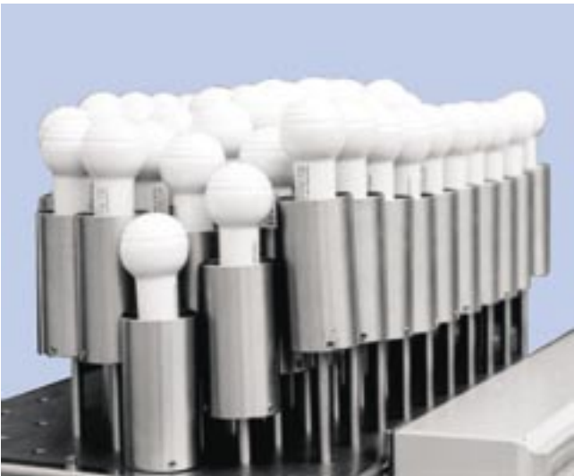
Figure 8: 3-D heating panel for laminating door trims
