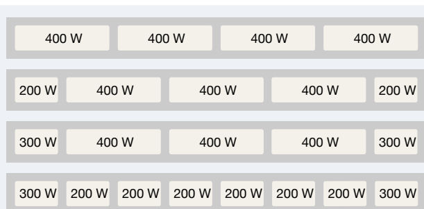
Fig. 64: Four examples of radiator equipment for an EBF/100 construction element
