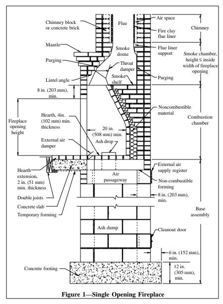
drops if there are air passage ways or ash pits incorporated into the base of the fireplace. If permanent forming is required at the top of the foundation walls, it must be a noncombustible material. Temporary wood forming is typically used to pour the hearth extension support. The forming should be placed so that the projected slab will meet a doubled wood floor joist, and be such that it can be easily removed.
